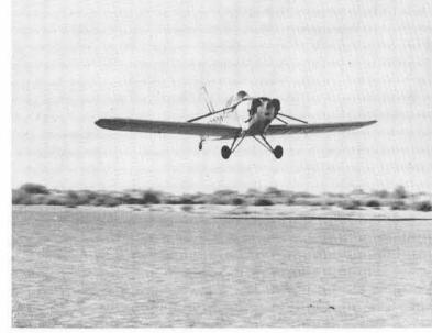
WHIZZING OVER the Seven-Bar runways, Lew Longmire logs more test time in his homebuilt airplane. Made of hardwood, plywood, fabric, and a little aluminum, the plane weighs only 750 lbs. with Lew and a full tank of gasoline aboard.
